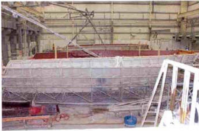
The first step in building the boat is the creation of the fiberglass hull. The entire boat, including the fiberglass, wood components and upholstery, is made at the plant.
