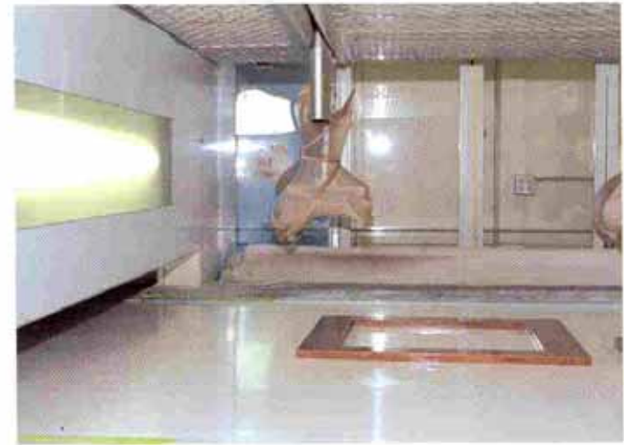
The Superfici flat-line finishing system scans parts so that spray heads only spray parts. The finish is a UV-cured waterbased product. Excess material is recycled and reused on the first three coats of the products.
