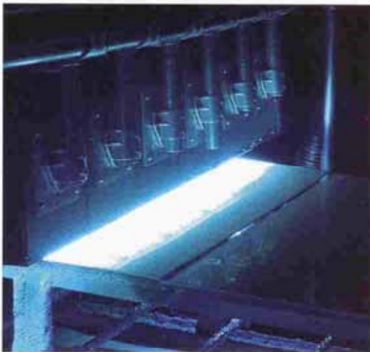
Wood marker boards with pigmented coatings are cured by a UV system.
