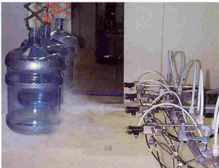
An abrasion-resistant UV clearcoat is automatically applied to water containers.
